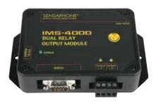
The IMS-4310 Dual Relay Output Module allows you to control two devices from any IMS-4000 Host or Node. Each output may be controlled either manually or automatically. Each output has the option of providing either a dry relay contact or 12VDC power. Two switches located inside the device select the output type.
