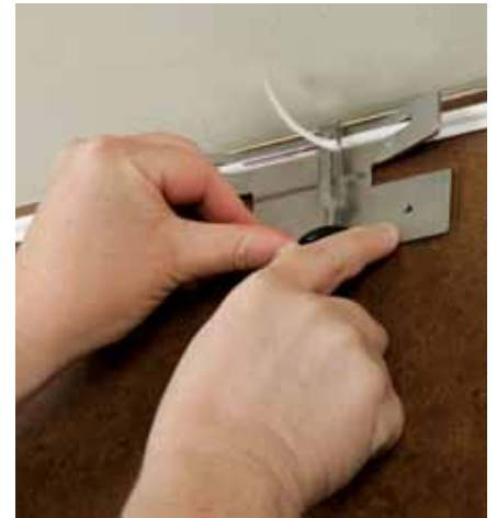
Window cut process using the 3M™ One Pass Window Cut Template WC-TEMP-20 and 3M™ One Pass Window Cut Tool WC-TOOL-50.
